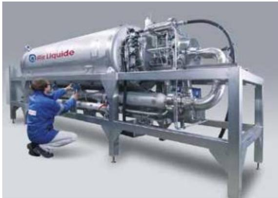
Up to 50 kW cooling power at 77 K
